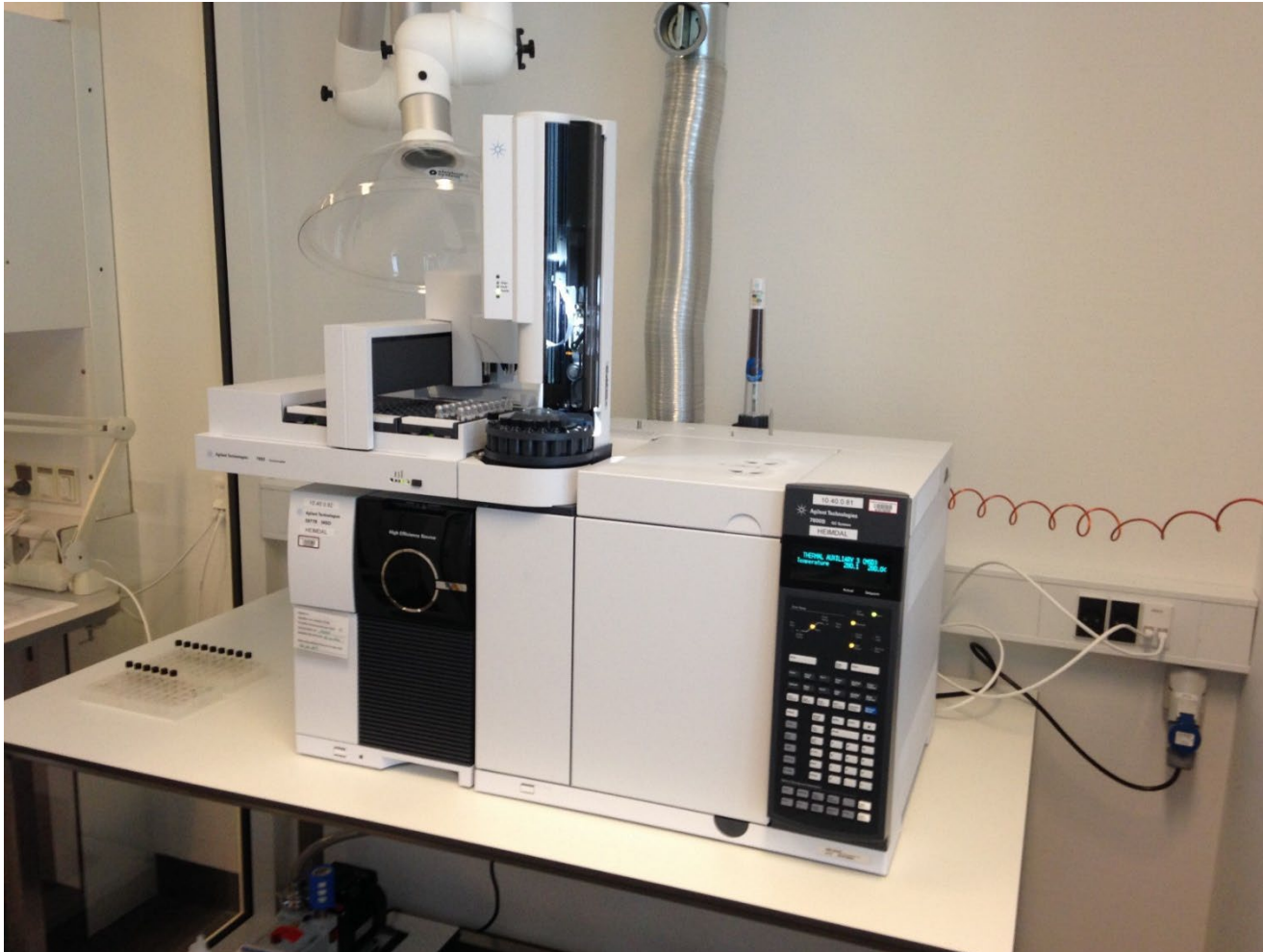
Agilent, single-Q, GC-MS system v/Klinisk Biokemisk Afdeling, Regionshospital Nordjylland
